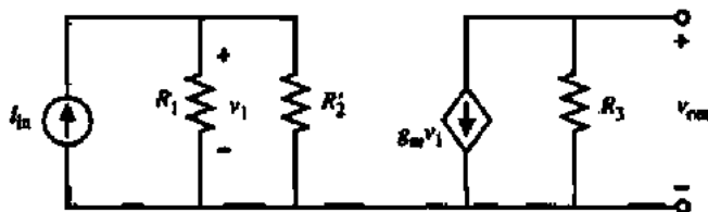
Figure A.1-12 The result of applying the Miller simplification concept.
