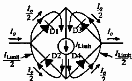
Figure 6.7-12 Macromodel for current limiting.
